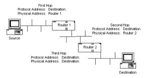
The relation between the destination host's protocol address and its physical address is obtained by the routers using the ARP request/reply mechanism, and the information is stored within the ARP table in the router (see "The ARP Table" on page 111).
